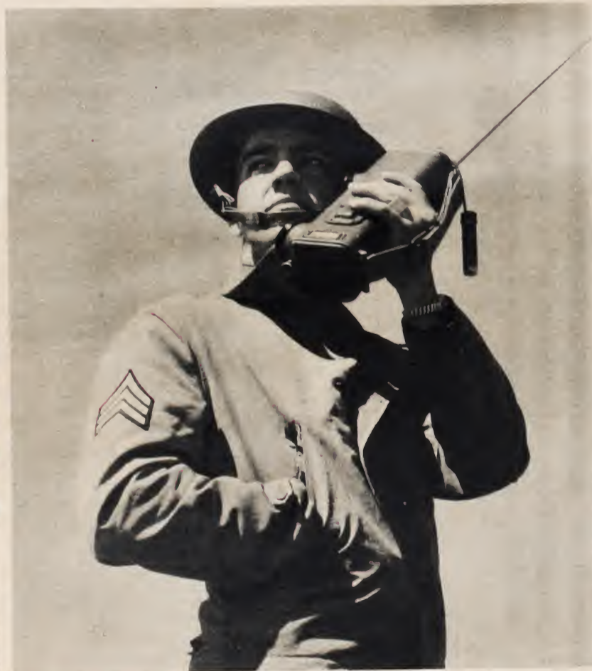
ON THE AIR. The Sergeant is operating a handy-talkie, a new hand set radio receiver and transmitter turned out by the Signal Corps. A push-to-talk button switches it from receiving to sending.
